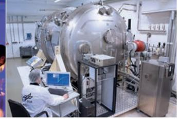
Space simulation facility for tests under vacuum and thermal boundary conditions
