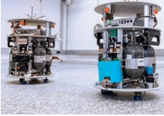
Test of control systems spacecraft docking in the Test Environment for Applications of Multiple Spacecraft (TEAMS) laboratory
