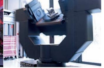
Verification and calibration of inertial sensors for spacecraft navigation in the GPS/INS laboratory
