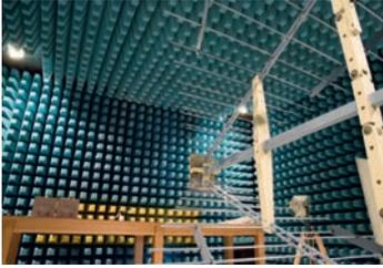
Electromagnetic compatibility (EMC) is checked for each system, and the tests are conducted in accordance with the usual EMC standards for everyday devices
