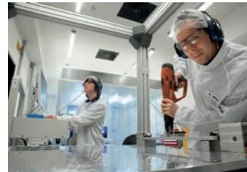
Shock tests on the pyroshock test rig
