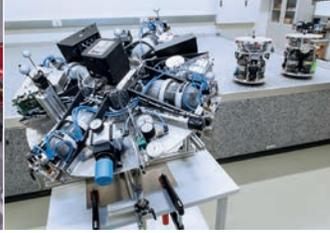
Simulating the movement of a satellite with five degrees of freedom to test control systems in the TEAMS laboratory
