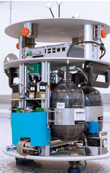
Test of Control Systems for Spacecraft Docking in the TEAMS Laboratory
