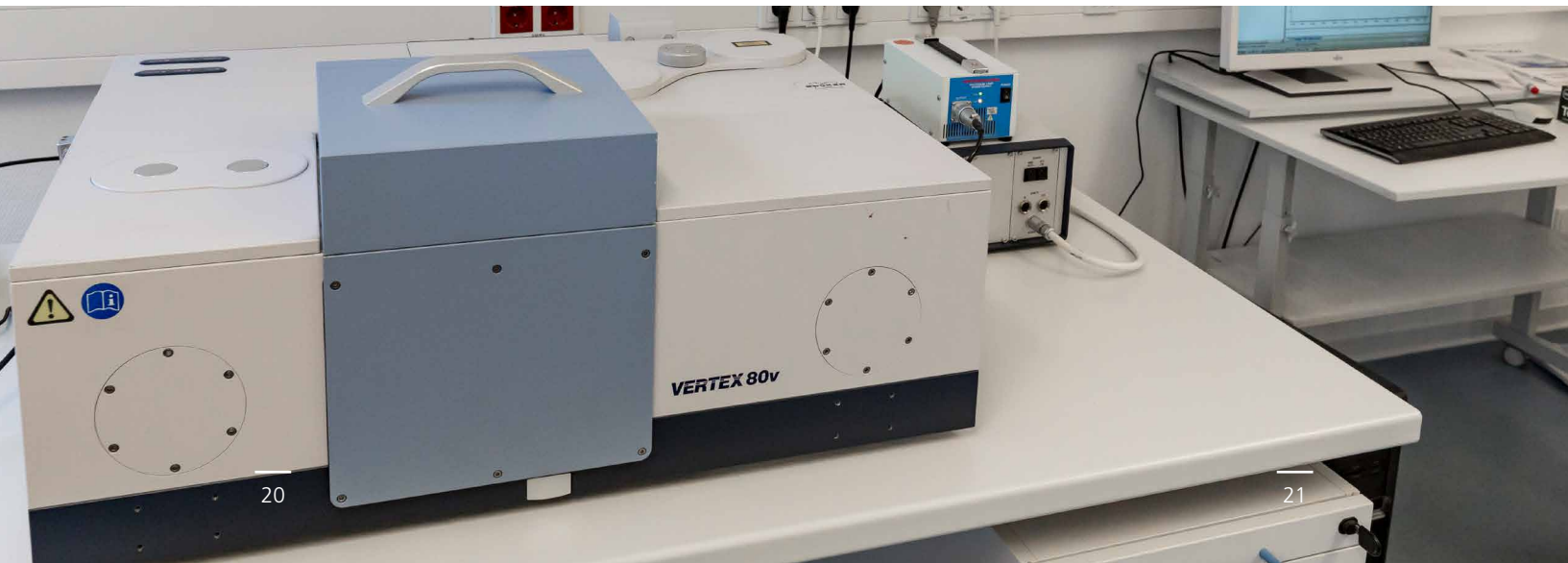
Spectrometer for the determination of thermo-optical properties
