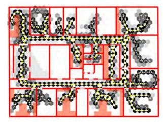
Iterative, Turbo-FeetSLAM: processing four data sets within the same building leads to much more encompassing maps. One can see how furniture is reflected by the map. (Scaled, rotated, and shifted to fit the known layout; resulting scale error roughly 0.5%).
