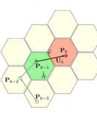
A portion of the hexagon grid and step transition U from time k to k-1. We assume that the step probability is conditionally independent of the pose history prior to  $P_{k-1}$ given knowledge of the Map (1st order Markov
