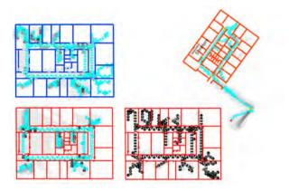
An example of four maps that result from four different walks in an office environment. (Scaled, rotated, and shifted to fit the known layout.)
