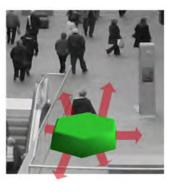
In our implementation of FootSLAM we adopt a 2D hexagonal grid for the Map which represents transition probabilities across edges of hexagons. Hexagons typically have a radius of 1/2 meter. The mapping part in the Rao-Blackwellized Particle Filter keeps track of the number of times an edge is crossed for each particle. The condi-
