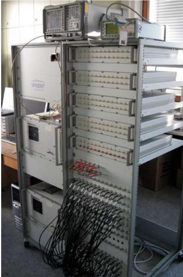
The picture shows the design of MASTER: the individual RF- and IF-outputs on the right hand side and GPS / Galileo simulator boxes on the left hand side
