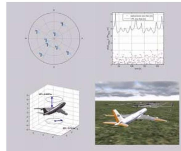
Automatic landing in a simulated Galileo+GBAS scenario
