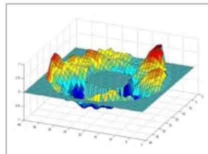
Distorted Wavefront, measured at a 1m Telescope
