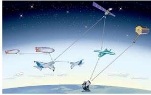
Application Scenarios for Mobile Optical Communications: From inter-satellite links to aeronautical links down to terrestrial scenarios
