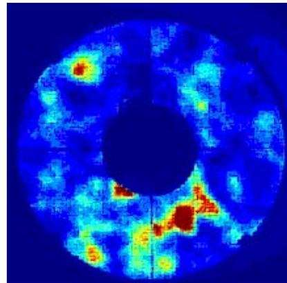
Scintillation Pattern caused by IRT
