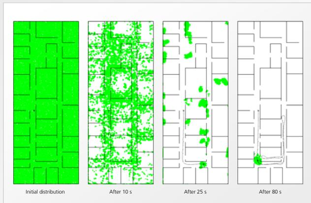
Integration with map-matching in the particle filter: A pedestrian wearing the foot-mounted sensor walked the indicated track (black line). At each figure the posterior position estimate (green) becomes increasingly accurate, after 80s it is unimodal.
