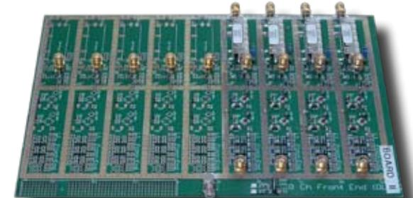
RF front end with four equipped channels
