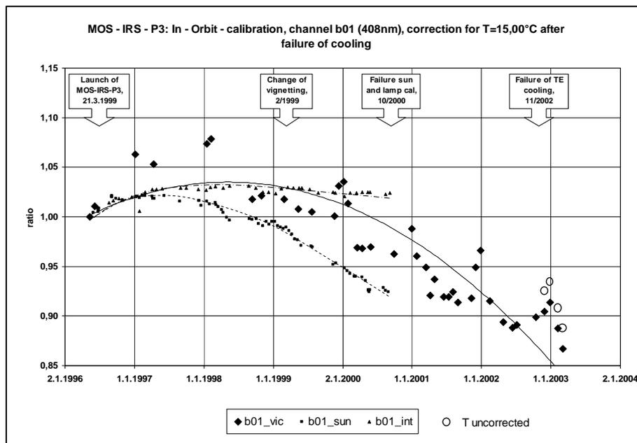
Fig. 2: Time trend of MOS in-orbit calibrations (vic: ground target based calibration, sun: sun calibration, int: internal lamp calibration), channel 01 (408nm)
