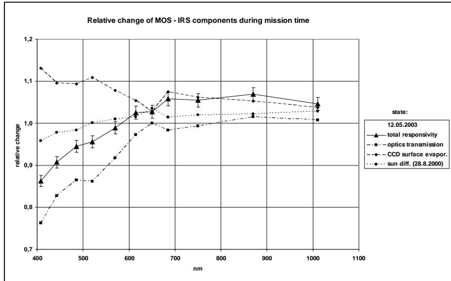
Fig. 5: Wavelength dependent change of optical and electronic MOS components in orbit
