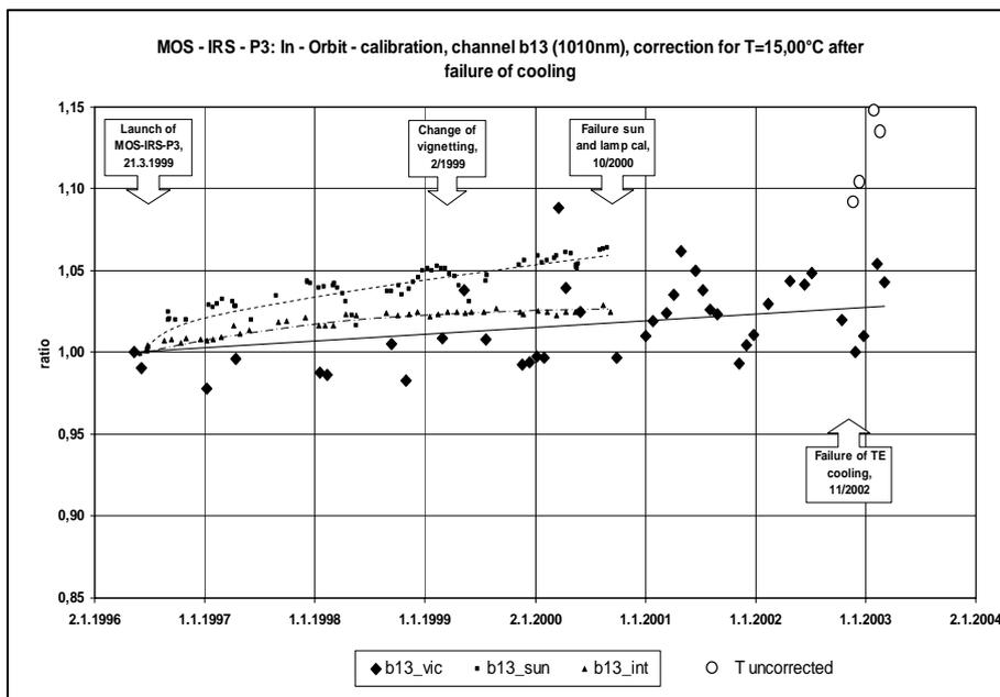
Fig. 4: Time trend of MOS in-orbit calibrations (vic: ground target based calibration, sun: sun calibration, int: internal lamp calibration), channel 13 (1010nm)
