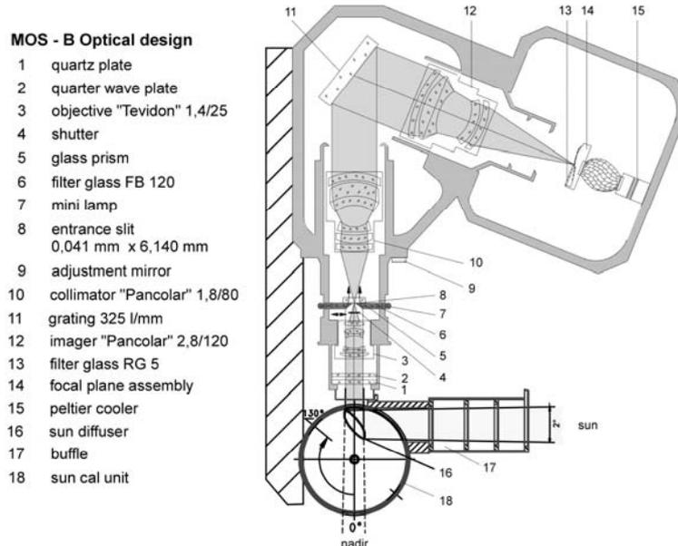
Fig. 1: Optical design and in-orbit calibration equipment MOS-B
