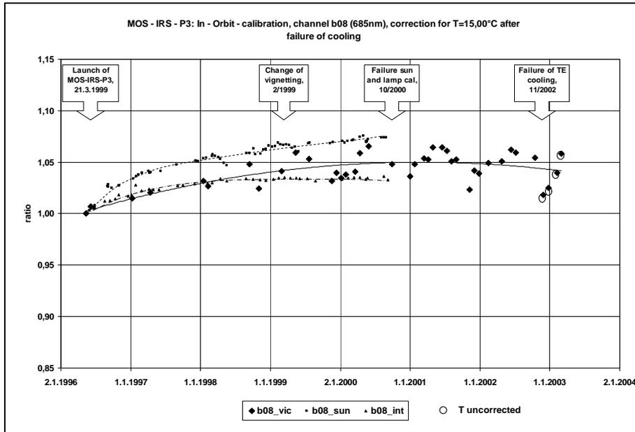
Fig. 3: Time trend of MOS in-orbit calibrations (vic: ground target based calibration, sun: sun calibration, int: internal lamp calibration), channel 08 (685nm)
