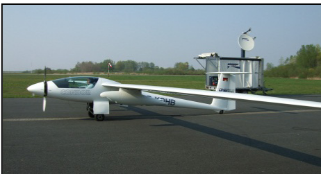
CONDOR (Stemme S10 aircraft), receiving antenna of OHB ARDS data link (back)
