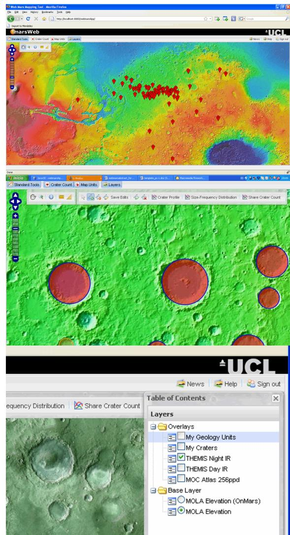
Figure 1. MarsWeb screenshots showing display of pre-existing craters (upper panel) and measured craters (red) superimposed on a hill-shaded and coloured MOLA DTM (using the USGS Flagstaff colour LUT). Other layers can be cascaded such as those from the J-Mars [4] WMS server shown here.
