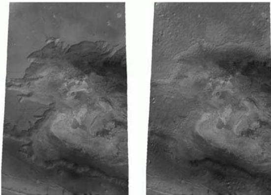
Figure 2: Part from the HRSC orbit 1235 (Valles Marineris): nadir image before (left) and after (right) photometric correction (Minnaert,  $k=0,5$ ).
