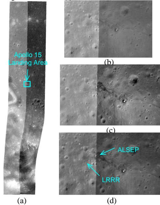
**Figure 3:** Comparison of orthorectified NACL and NACR image pair. (a) Orthorectified image pair showing the Apollo 15 landing area, (b) a close-up view in the orthorectified image pair generated using the standard SPICE kernels, (c) using the temperature-dependent kernels, and (d) after boresight calibration.
