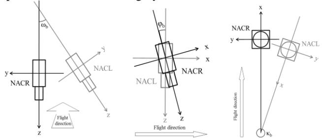
**Figure 1:** Conceptual illustration of the angular boresight offsets: omega  $\omega_b$  (left), phi  $\phi_b$  (middle), and kappa  $\kappa_b$  (right).
