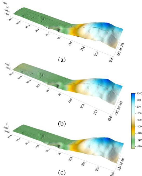
**Figure 2:** DEMs generated from NAC images at Apollo 15 landing site: (a) using the standard SPICE kernels, (b) using the temperature-dependent SPICE kernels, and (c) after boresight calibration.
