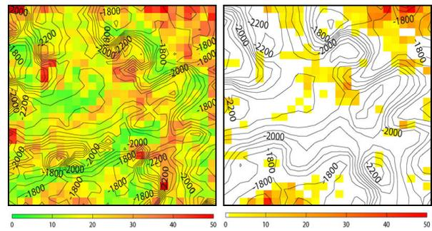
**Fig. 3:** Height RMS’ in [m] from Facets Stereo Vision. Left: Calculation without any filtering (cp. Fig. 1a). Right: RMS increase after image smoothing, carried out with 3x3 DTM filtering (cp. Figs. 1c and 2, right).
