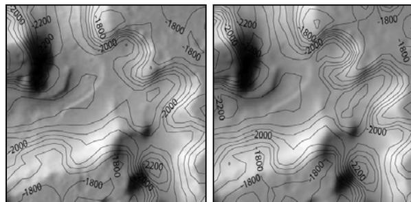
**Fig. 2:** Facets Stereo Vision results from smoothed images and 3x3 DTM filtering after each iteration (cp. Fig. 1c). Left: Gaussian filter,  $\sigma = 0.75$ . Right: Gaussian filter,  $\sigma = 1.5$ .
