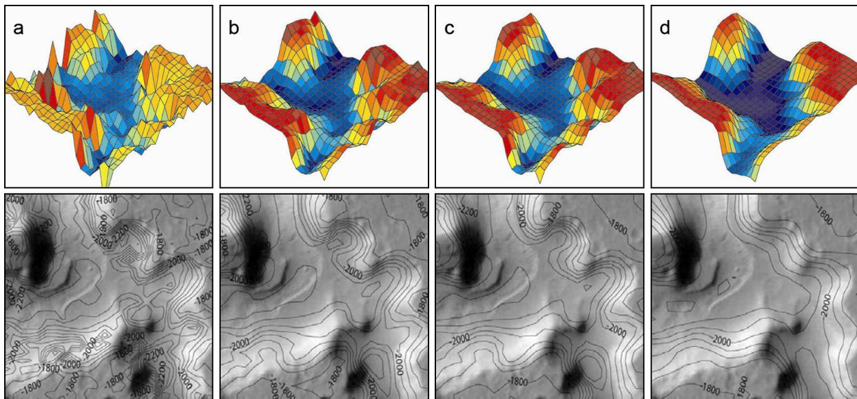
**Fig. 1:** Results of Facets Stereo Vision – Perspective DTM views and orthoimages with derived contour lines: a) Calculation with no DTM filtering, b) 3x3 median filtering after each step, i.e., applied to the final DTM of a particular facet size, c) 3x3 median filtering after every least squares iteration, d) 5x5 median filtering after every least squares iteration.
