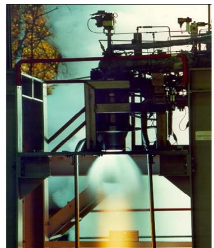
Steam generator combustion chamber test
