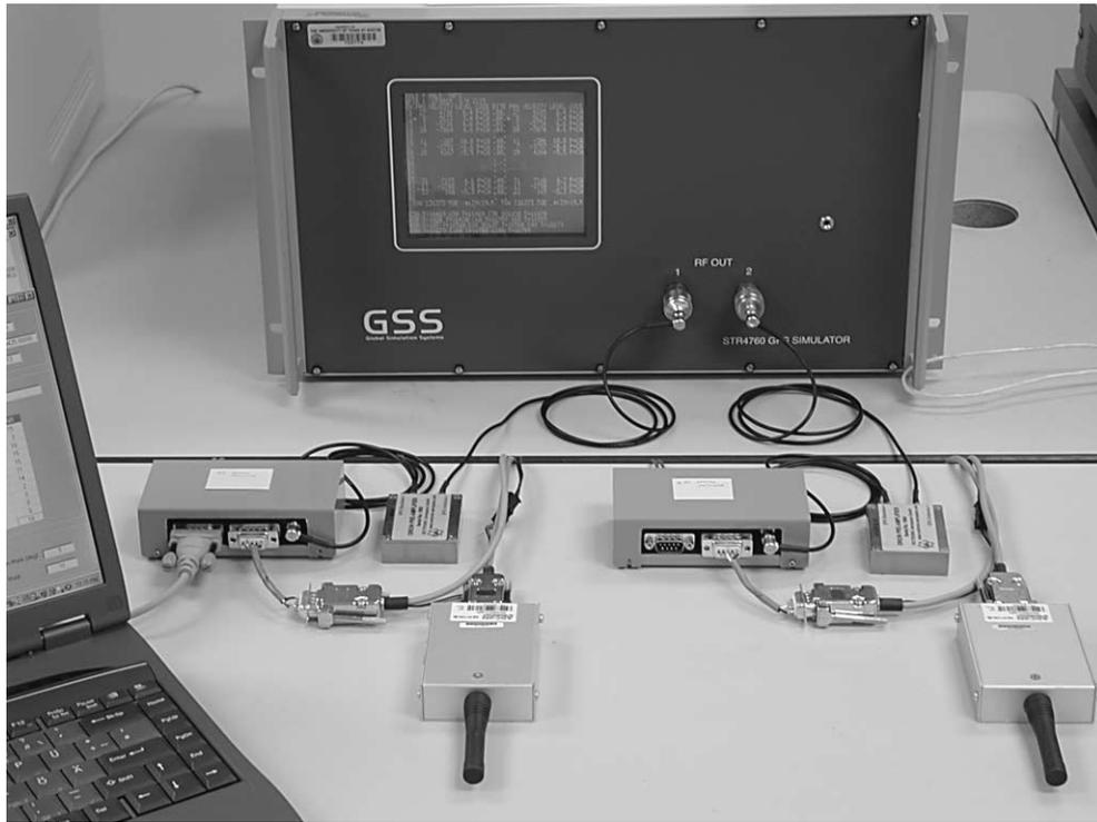
Fig. 5. Formation flying simulation setup showing the STR4760 signal simulator, two Orion GPS receivers with external preamplifiers (VAS Aerospace) and a host PC attached to one receiver for configuration and data recording. The data exchange between the auxiliary data ports is performed via two UHF radio modems (ADCON).
