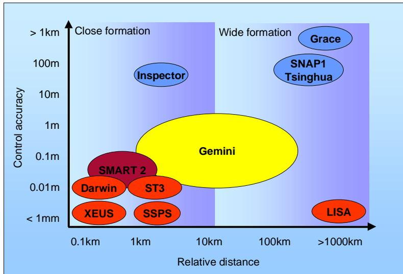
Fig.1 Formation Flying Control Accuracy versus distance for selected missions
