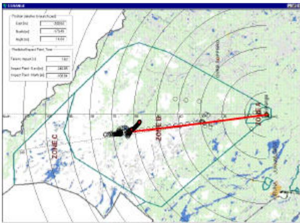
**Fig. 15** Screenshot of the Instantaneous Impact Point (IIP) prediction display. Ground track (line) and IIP (circles) for the TestMaxus-4 flight.
