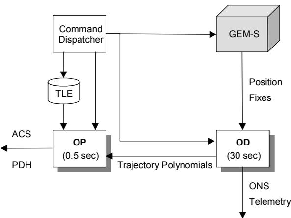
**Fig. 3** Schematic view of the ONS architecture. Software threads are indicated by shaded boxes.
