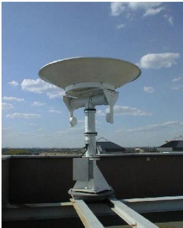
**Fig. 6** DLR's experimental ground station will receive GPS based twoline elements from BIRD to allow autonomous pass predictions and antenna pointing
