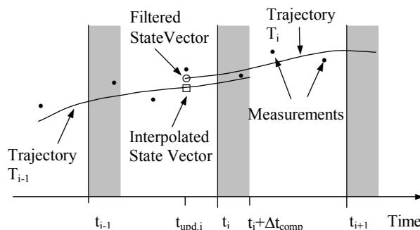
**Fig. 2** Timeline of the BIRD real-time navigation process. Shaded bars indicate computational activity.
