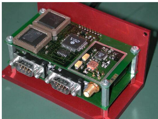
Fig. 1 The Mitel ORION receiver comprises a main receiver board (top) with RF front end, correlator, processor and memory as well as an interface board with power regulator, battery backup and serial interfaces (bottom). Physical dimensions are 95 x 50 x 30 mm 3 .
