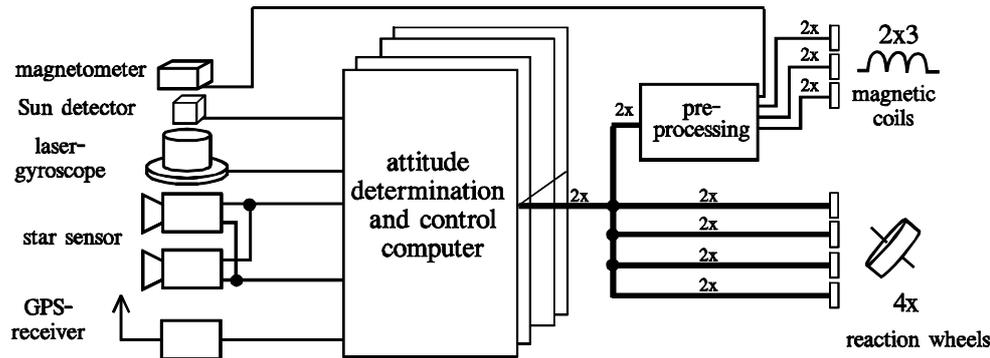
Fig. 2 Block scheme of the ACS system
