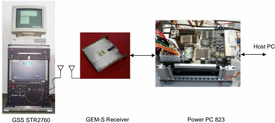
**Fig. 4** Hardware-in-the-Loop simulation scenario for verification of the ONS software.
