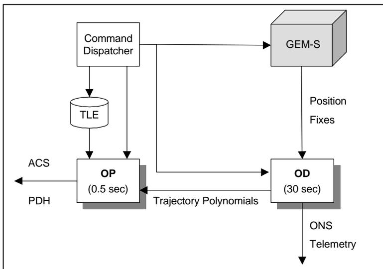
Fig. 3 Schematic view of the ONS architecture. Software threads are indicated by shaded boxes.
