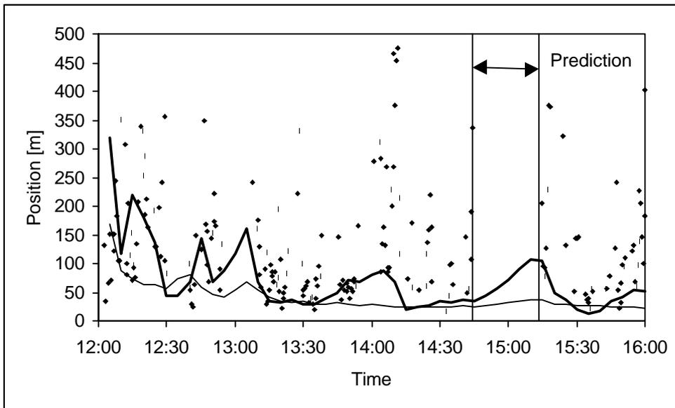
**Fig. 5** ONS performance from hardware-in-the-loop simulations with a four hour GEM-S data set. The bold line indicates the difference of the ONS filter results and a precise reference trajectory. The thin line indicates the position variance of the filter, while the measurement residuals are marked as diamonds.
