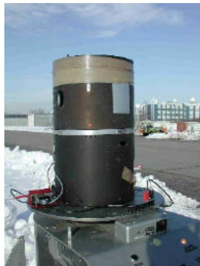
**Fig. 2** Turn table with Test Maxus-4 service module and Orion GPS receiver for assessment of the dual blade antenna system
