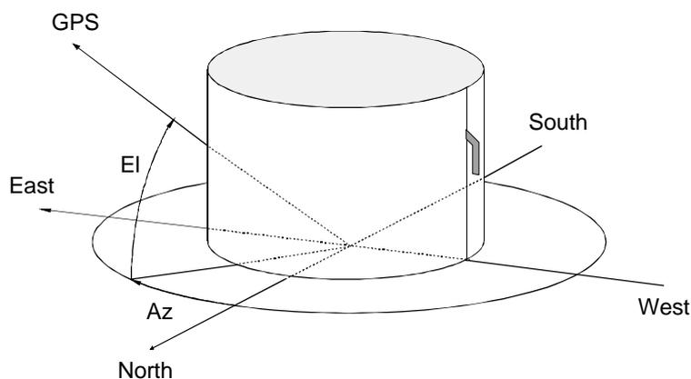
**Fig. 3** Test setup for measuring the blade antenna diagram using real GPS signals
