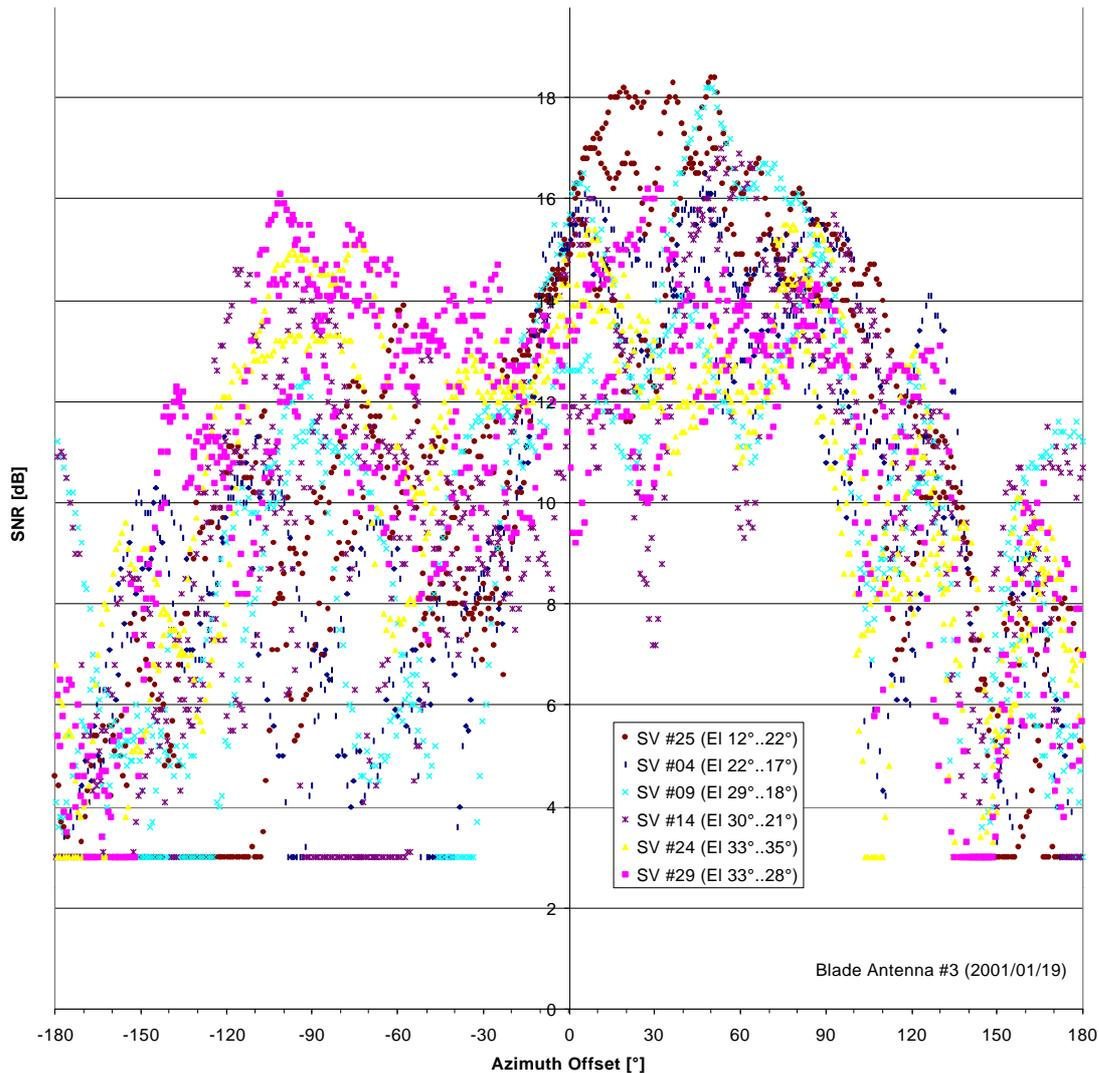
**Fig. 4** Azimuth variation of a single blade antenna (model #3) for low elevation angles (12° to 35°)
