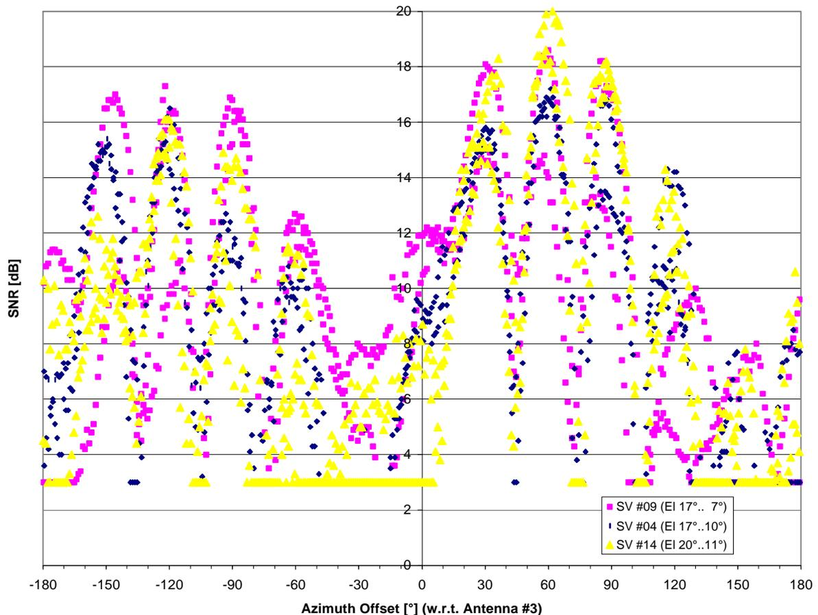
**Fig. 6** Signal interference for dual antenna configuration with  $2\lambda$  baseline
