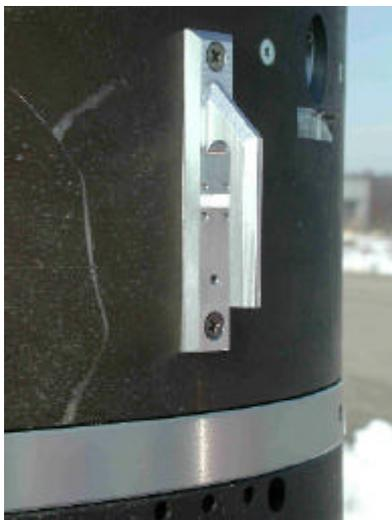
**Fig. 1** Blade antenna for GPS L1 frequency attached to 14" service module of the Test Maxus-4 flight
