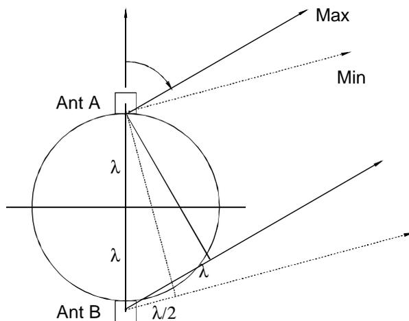
**Fig. 5** Signal interference for dual antenna configuration with  $2\lambda$  baseline
