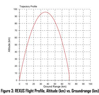
During the descent phase in the lower atmosphere, at an altitude of about 26 km, the payload is decelerated with a maximum acceleration of about 6 g. The recovery sequence is initiated after about 7 minutes of flight, at an altitude of about 5 km. A parachute system decelerates the payload to a terminal velocity of ~10 m/s before landing.
