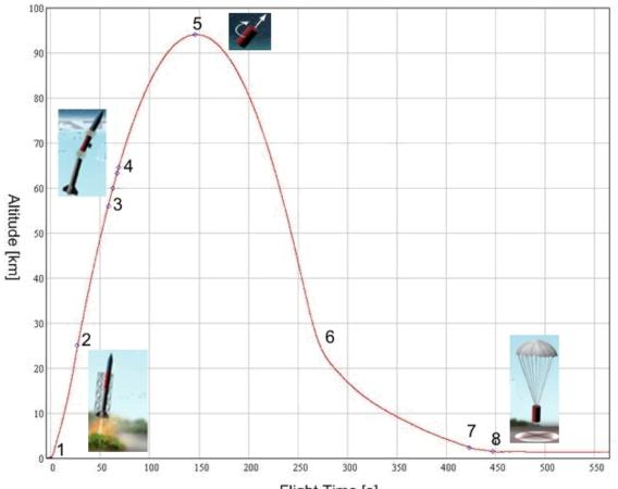
Flight Time [s] Figure 4: REXUS Flight Profile, Altitude (km) vs. Flight Time (s), Flight Events
