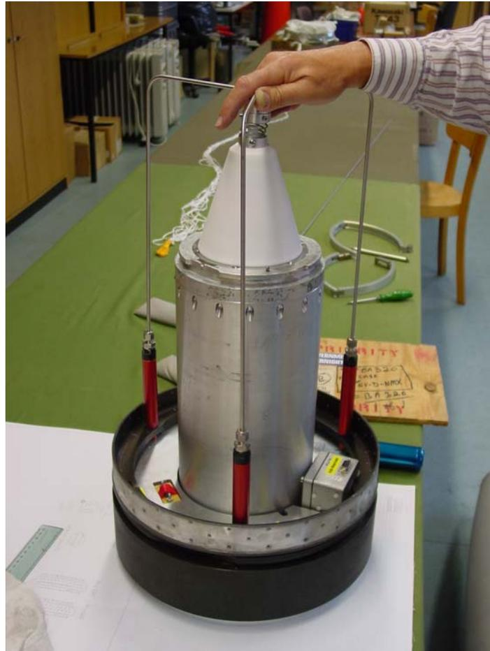
**Figure 7: Example of an Experiment situated below the Nosecone**
