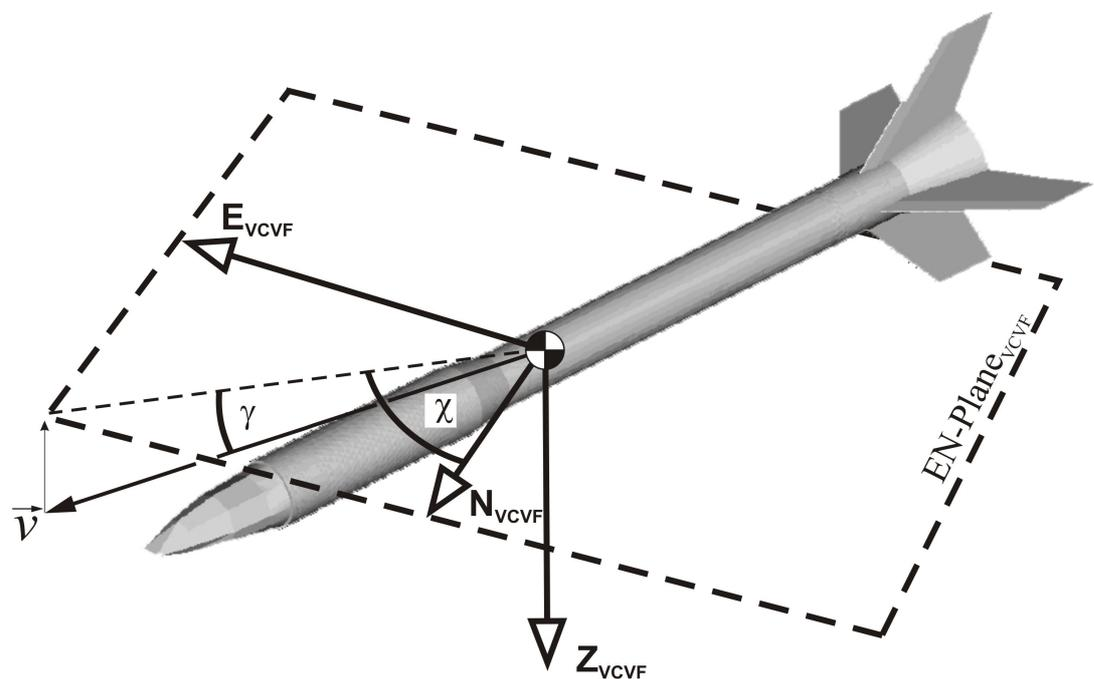
Figure 9-6: Flight Path Angle and Heading Angle
