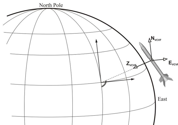
Figure 9-5: Vehicle Carried Vertical Frame
