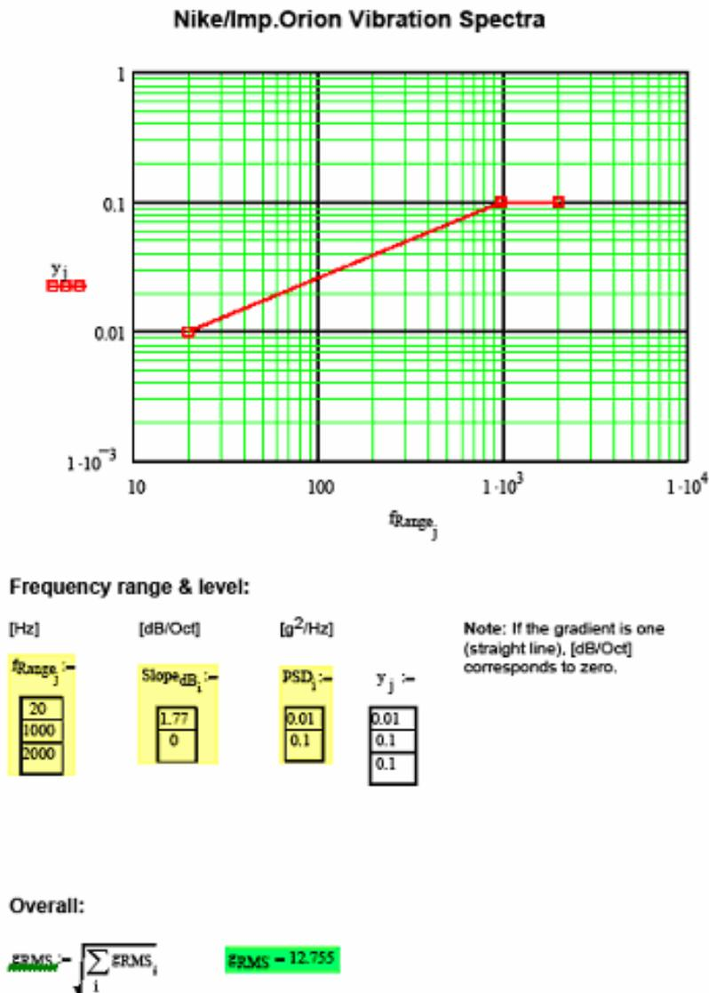
Figure 6-1: Nike-Imp.Orion Vibration Spectra
