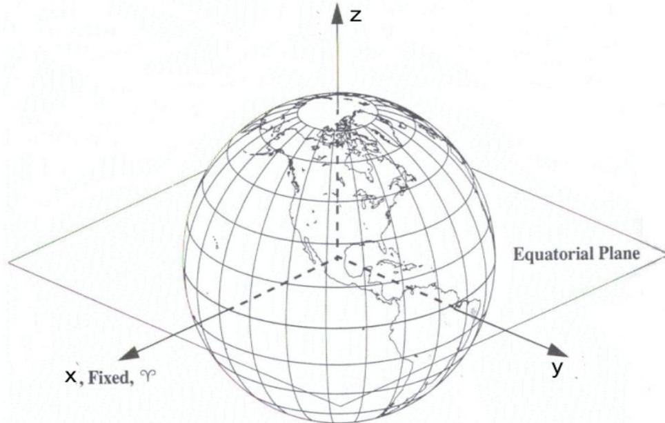
**Figure 9-1: Earth-Centered Inertial System (ECI) [Ref. [5]]**
