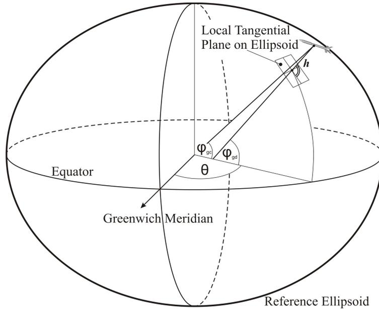
**Figure 9-3: WGS84 Reference Ellipsoid**
