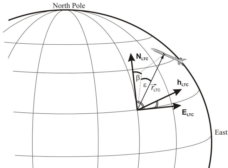
**Figure 9-4: Local Tangent Coordinate System (LTC)**
