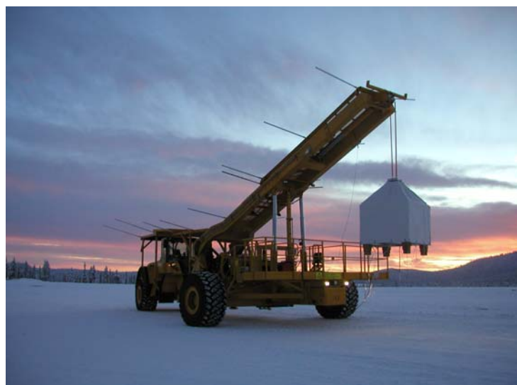
Fig. 2: Hercules launch truck with Payload Gondola
