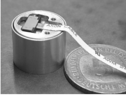
Figure 7. Six dimensional force torque sensor in fingertip.
