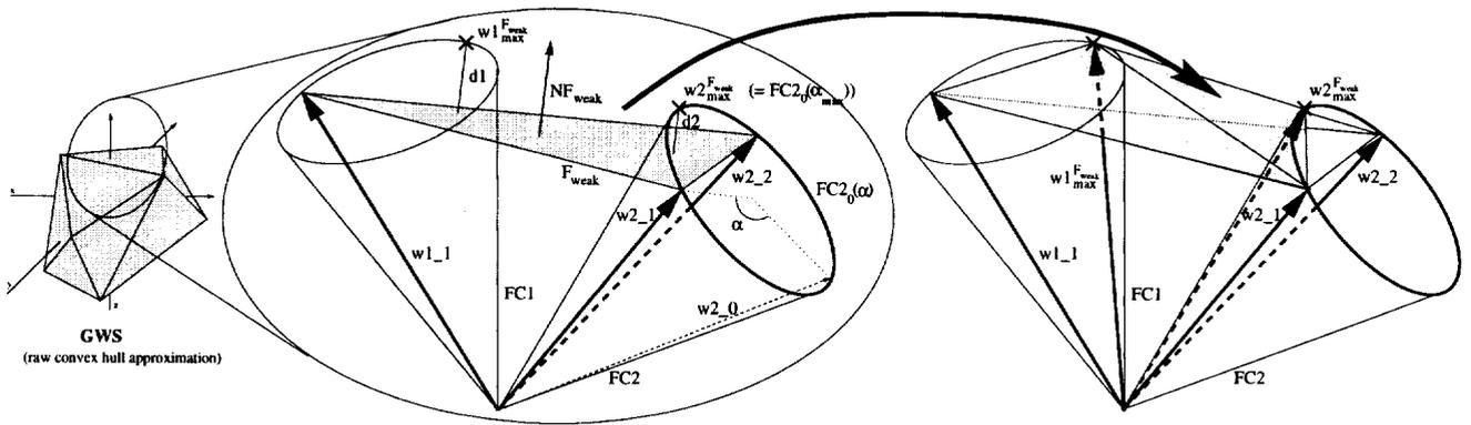
Figure 3: Improving friction cone approximation at the weakest convex hull face, 3D analog of 6D case
