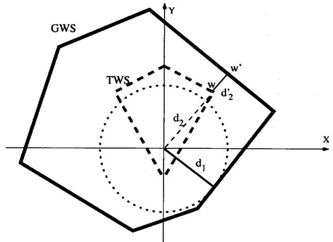
Figure 2: Quality measure with (dashed line) and without a given task wrench space (dotted)
