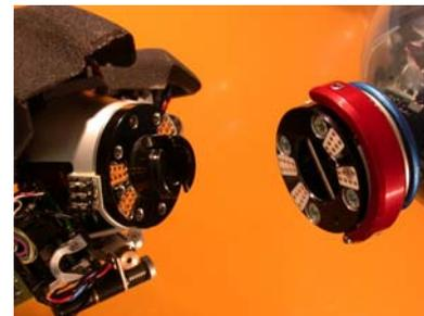
Fig. 5: Customized tool adapter
