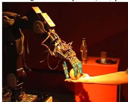
*Fig. 8: Tracking and grasping an object.*
