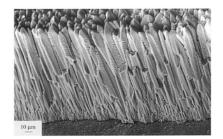
Ceramic coating on a compressor blade
