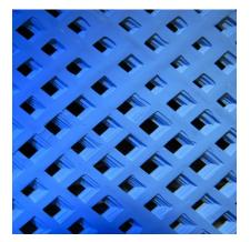
Ceramic fibres: detail of a WHIPOX™ plate
