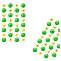
lonic bonds (e.g. salt or ceramic): breaks under strain. These materials are very hard, but brittle.
