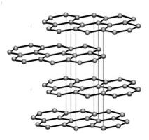
Covalent bonds (e.g. graphite): Atoms within one layer are bonded together and cannot be separated easily. Different layers can however be moved across each other.
