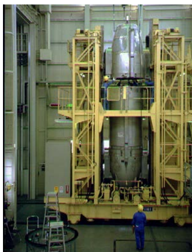
Drop capsule in Japanese Microgravity Center Kamisunagawa
