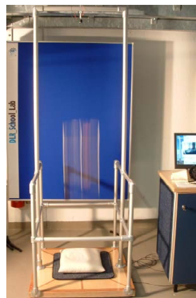
The miniature drop tower in the DLR_School_Lab Köln
