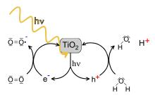
Photocatalytic reaction with titanium dioxide
