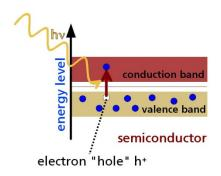
Diagram of the energy- band- model of semiconductors and the excitation through light energy  $(h\nu)$
