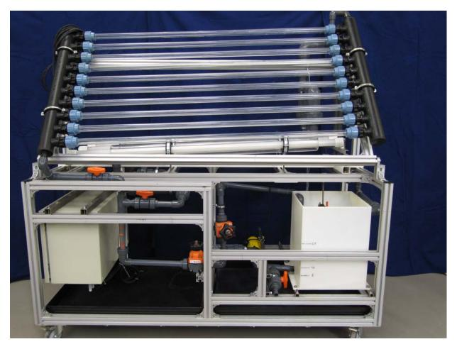
The apparatus for solar water purification in the DLR\_School\_Lab Cologne combines two reactors: The ten sloping tubes can be used to carry out the experiment using sunlight. Underneath, three almost horizontal tubes carry the chemicals when artificial UV light is used. The bottom of the apparatus carries (from left to right) a switchboard, valves, the pump (yellow) and tank for the reactants.
