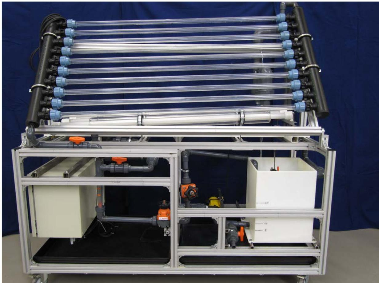
The apparatus for solar water purification in the DLR\_School\_Lab Cologne combines two reactors: The ten sloping tubes can be used to carry out the experiment using sunlight. Underneath, three almost horizontal tubes carry the chemicals when artificial UV light is used. The bottom of the apparatus carries (from left to right) a switchboard, valves, the pump (yellow) and tank for the reactants.
