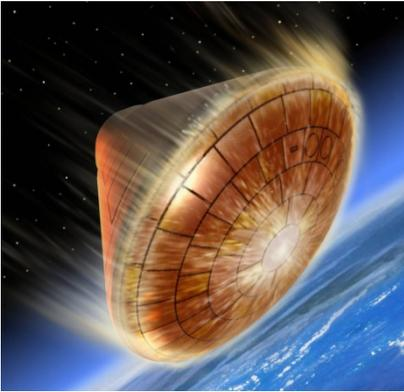
When re-entering the Earth's atmosphere, heat shields have to be able to withstand temperatures of up to 5,000°C. That is as hot as the surface temperature of the Sun!
