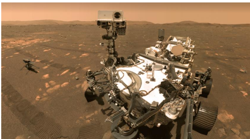
Similar to its predecessor, the Mars rover Perseverance weighs almost a tonne and has the size of a small car. It transported a small helicopter to Mars, which – despite the very thin Martian atmosphere – succeeded in making the first flight on an alien celestial body. (Image: NASA)
