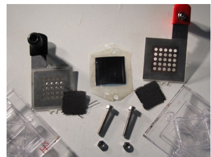
Fig. 4: Components of a simple fuel cell
