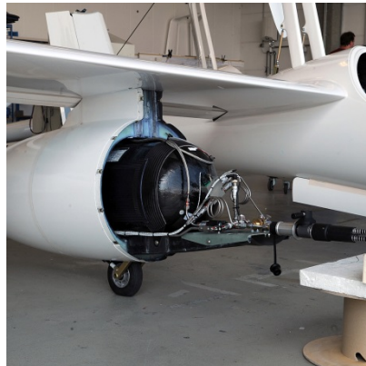
Fig. 9: ANTARES filling up on hydrogen
