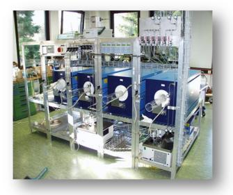
**COSTA:** COrrosion test stand for STagnant liquid lead Alloys
