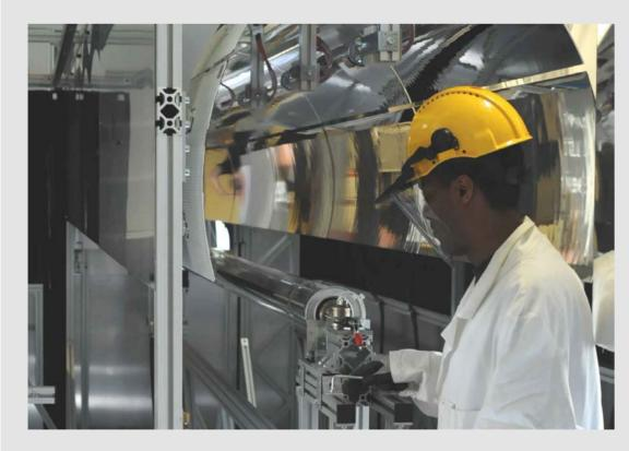
Figure 2: Linear focus solar simulator
