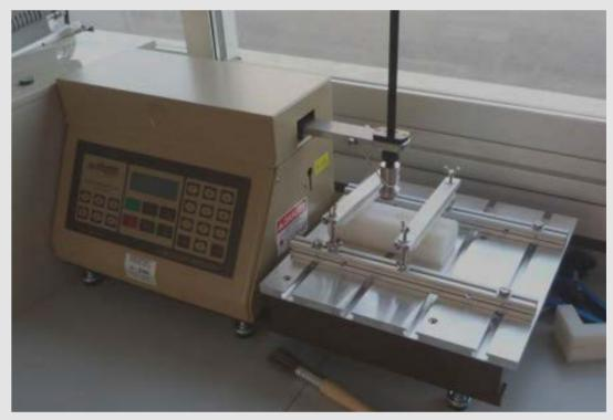
Figure 6: Taber Linear Abrasion Test for AR-coating testing
