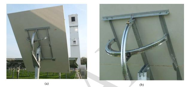
FIGURE 5. (a): First rim drive prototype with 8 m<sup>2</sup> mirror surface mounted at Solar Tower Jülich, Germany (without drive units); (b): Detail.
