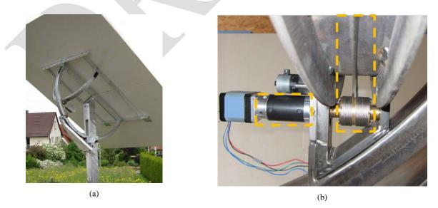
FIGURE 1. (a): First rim cable drive prototype with 8 m<sup>2</sup> mirror surface; (b): Cable drive system with intermediate gear in the left and winch wheel in the right dashed box.
