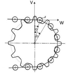
FIGURE 2. Example of different positions between chain rollers and sprocket teeth and angles for calculation of a polygon effect [5].
