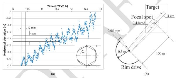
FIGURE 3. (a): Fluctuating focal spot due to polygon effect. (b): Change of angle of drive and surface normal.
