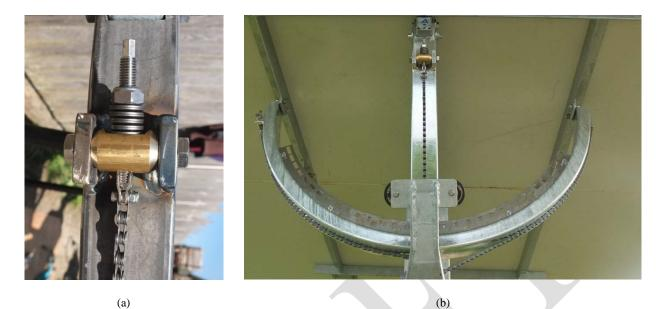
FIGURE 3. (a): Pretensioning in the rim gear stage by compressing disc springs with nuts. (b): Arrangement of rim chains with pretension mechanism
