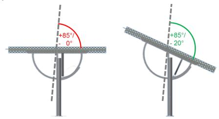
Fig. 8. Angle range limits of primary axis for central 2. rim (left) and for shifted 2. rim (right)
