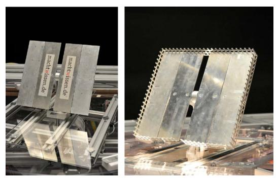
Fig. 2. Left: Isolated heliostat model, mounted on six component balance in wind tunnel. Right: heliostat with edge manipulator (academic test case)
