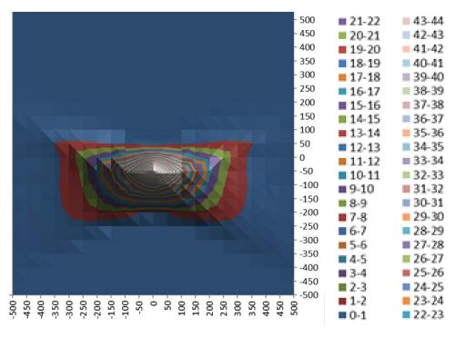
Fig. 9. Losses due to reduced angle range of primary axis (+85°/-0°) as percentage of annual energy yield, tower height 120m (position 0m/0m), optimized orientations of horizontal primary axis
