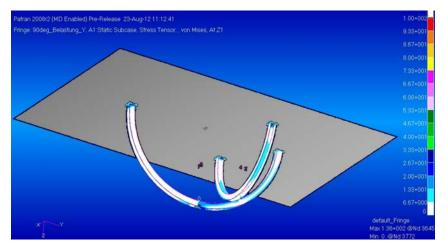
Fig. 12. FEM-analysis of tension in rims at storm conditions
