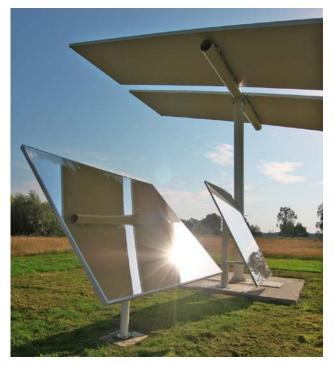
Fig. 4. Laminated mirror facets for heliostats
