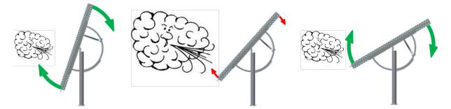
Fig. 13. Speed adaption according load to reduce motor size and to avoid self-locking gears of low efficiency
