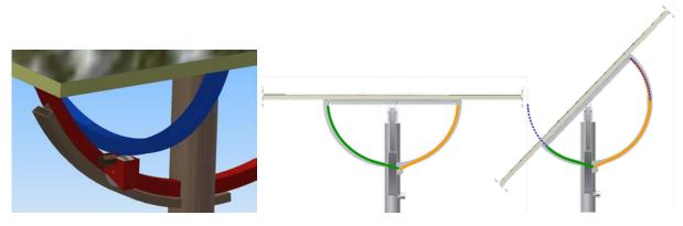
Fig. 7. Winch wheels with rims: Length change of cables of both directions during rotation is equal and thus speed when leaded on the same circular path realized by rims
