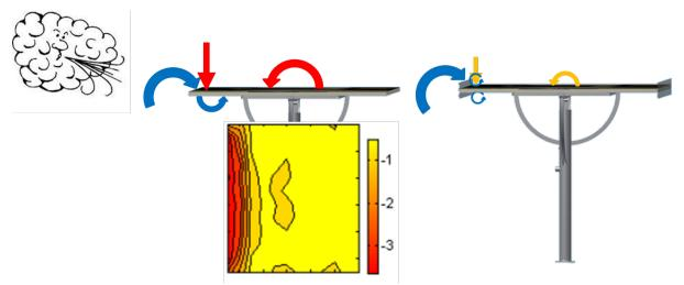
Fig. 3. Left: Turbulences causing high pressure coefficients at the frontal edge [15] and high overturning moment at storm conditions with heliostat in stow position. Right: Manipulators reducing suction and overturning moment
