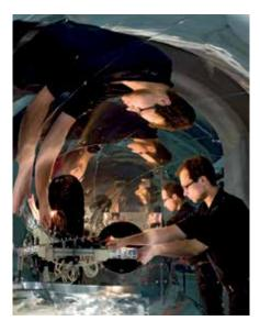
Special test rigs at the QUARZ Center measure the optical characteristics of the receivers, absorber tubes and solar mirrors.
