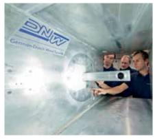
Preparation for a wind tunnel test to measure convective heat loss in a solar tower model.
