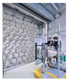
Synlight is equipped with three radiation test chambers. In the first series of experiments conducted at the facility, DLR scientists are testing processes for the solar generation of hydrogen. Image: DLR/Hauschild
