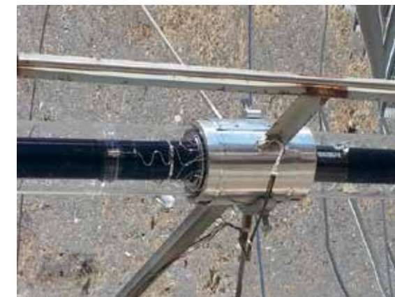
Figure 3: DLR measurement receiver with six temperature sensors on circumference (see A - F in Figure 4) and one sensor in the fluid.
