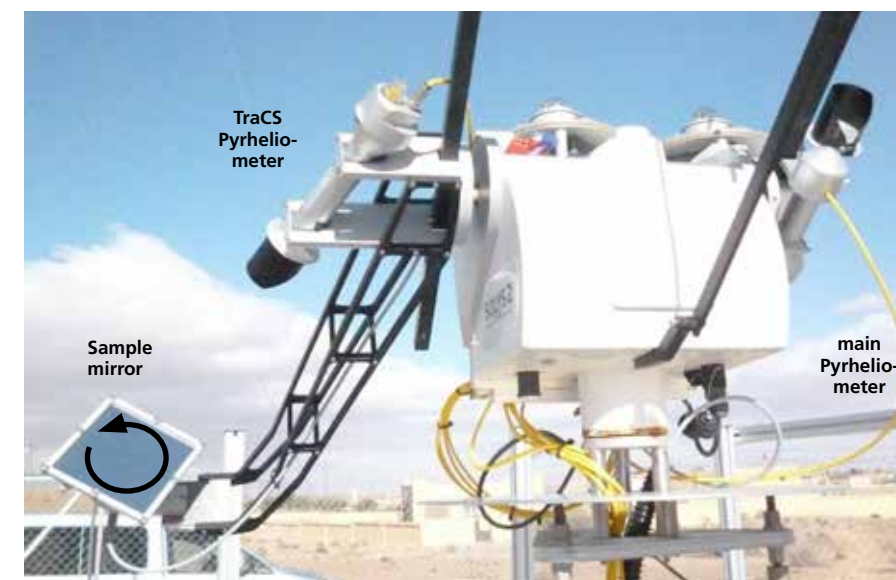
Figure 2: Tracked cleanliness sensor (TraCS) for real-time on site cleanliness measurement.
