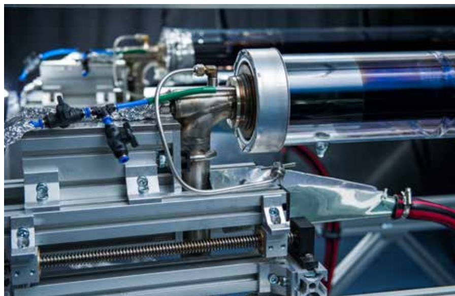
Part of test bench to measure the optical efficiency of parabolic trough receivers.
