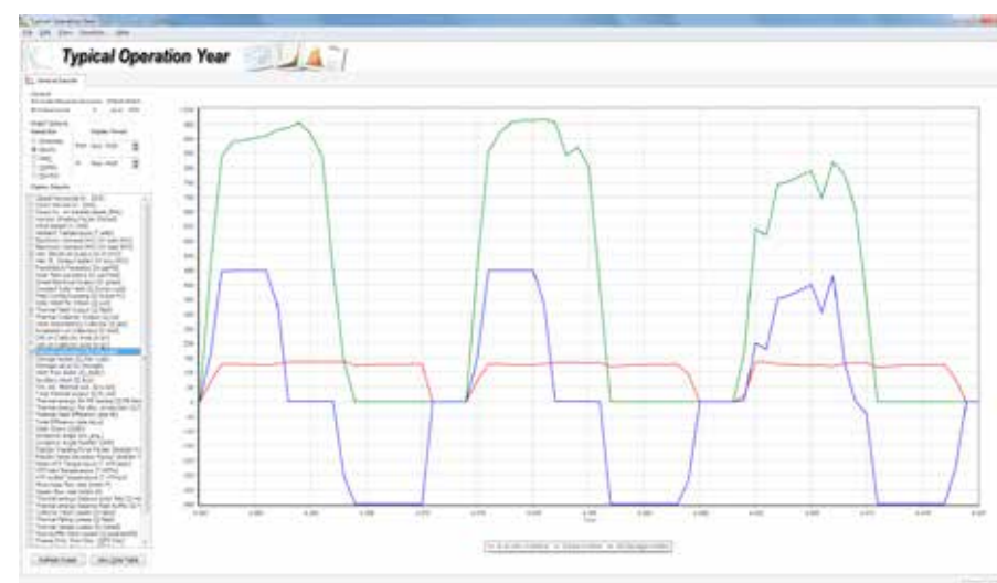
Figure 2: Visualisation of greenius results for three days showing the operation of a parabolic trough CSP plant.
