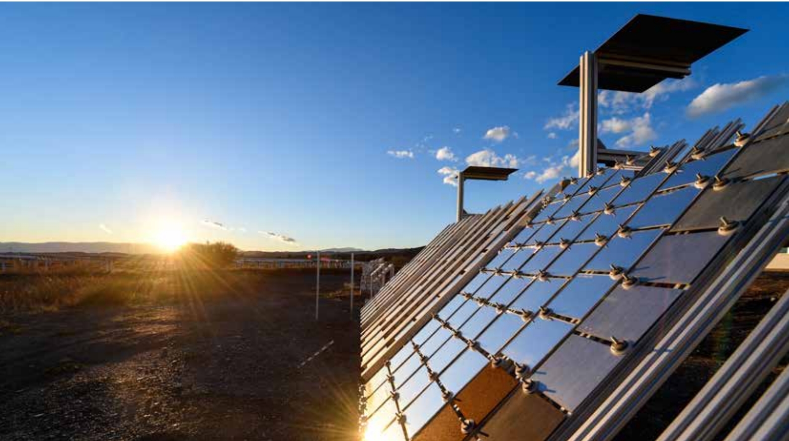
Figure 1: Outdoor exposure testing of solar reflector samples at CIEMAT's PSA.
