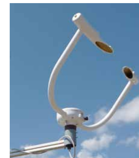
Figure 3: FS11 Scatterometer to derive extinction rate.
