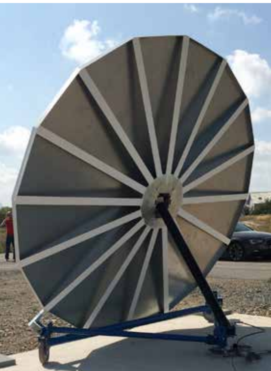
Figure 1: 8 m 2 prototype of low cost carousel heliostat with monolithic sandwich concentrator.
