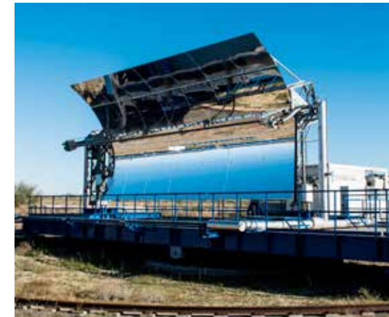
KONTAS rotating platform for performance testing of components at PSA.
