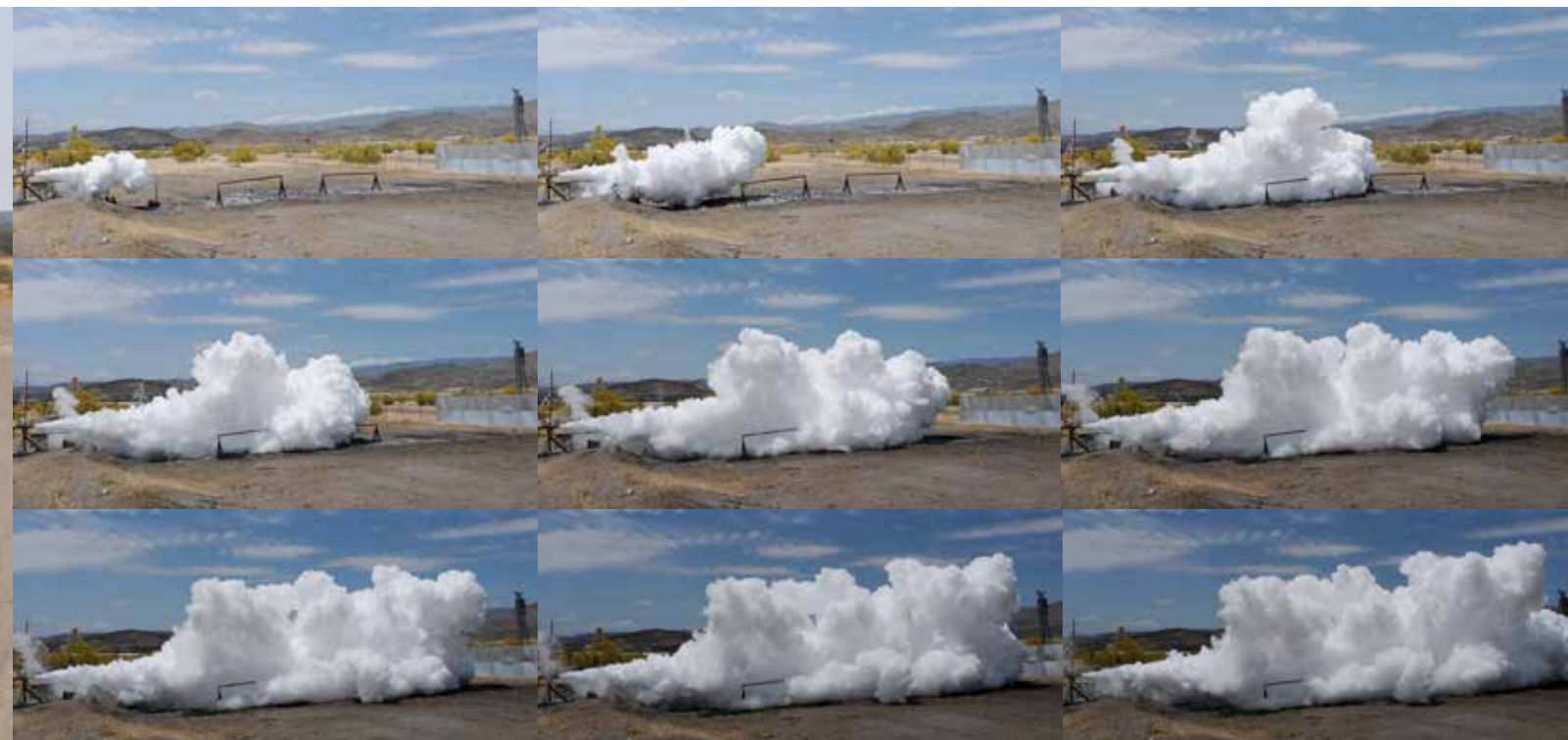
Figure 4: Photo series taken during the first 3 seconds (3 pictures/second) of the 2" HELISOL® 5A release test at 420°C
