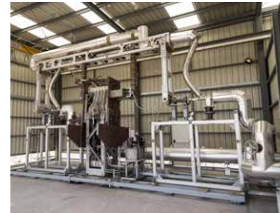
REPA test bench to test flexible connections for parabolic troughs.
