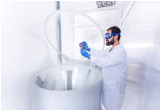
Figure 2: Salt spray testing of reflector samples according to ISO 9227 to accelerate silver corrosion processes.
