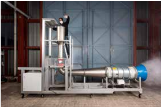
Figure 3: Custom-made sand erosion chamber to mimic sand and dust storms.
