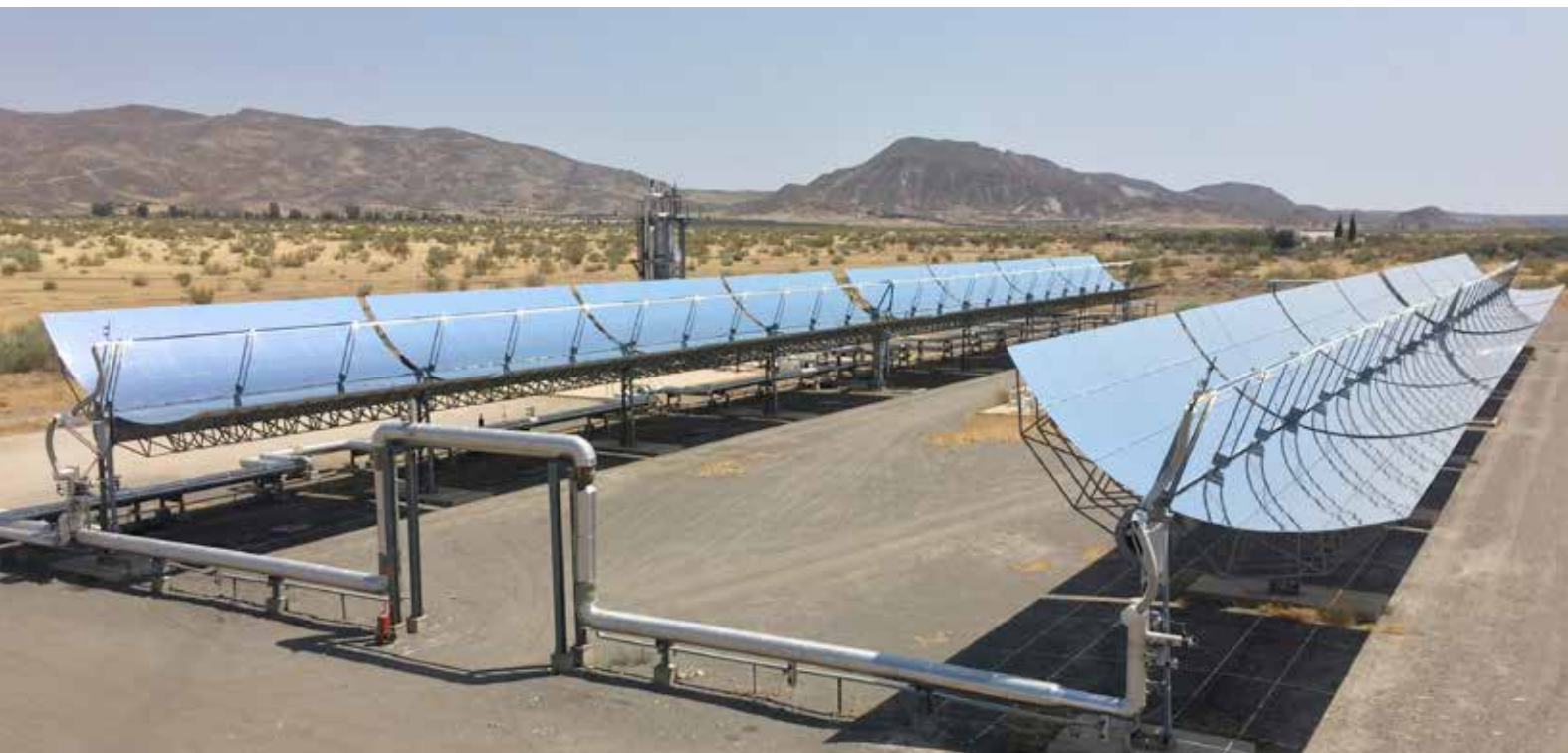
Figure 3: Ciemat's PROMETEO test facility at PSA for technical studies on silicone based heat transfer fluids.
