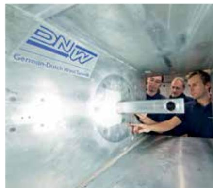
Preparation for a wind tunnel test to measure convective heat loss in a solar tower model.
