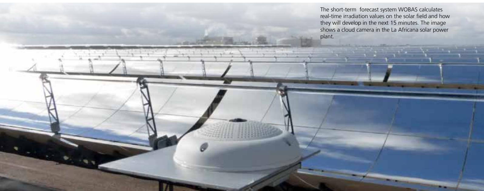
The short-term forecast system WOBAS calculates real-time irradiation values on the solar field and how they will develop in the next 15 minutes. The image shows a cloud camera in the La Africana solar power plant.
