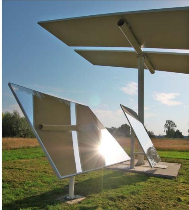
**Fig. 4. Laminated mirror facets for heliostats**
