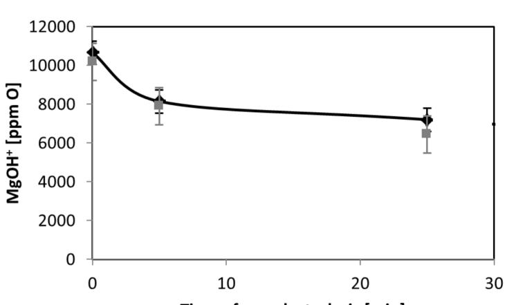
Time of pre-electrolysis [min] Figure 4: Concentrations of corrosive impurity MgOH<sup>+</sup> in molten salt over the time of PE determined with the CV (black curve) and acid consumption (grey points) method, respectively.
