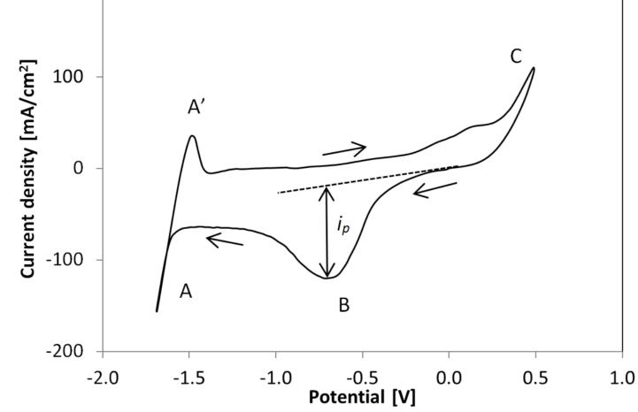
Figure 2: Cyclic voltammogram obtained on a tungsten electrode in the eutectic MgCl<sub>2</sub>/KCl/NaCl at 500 °C. Sweep rate v: 200
