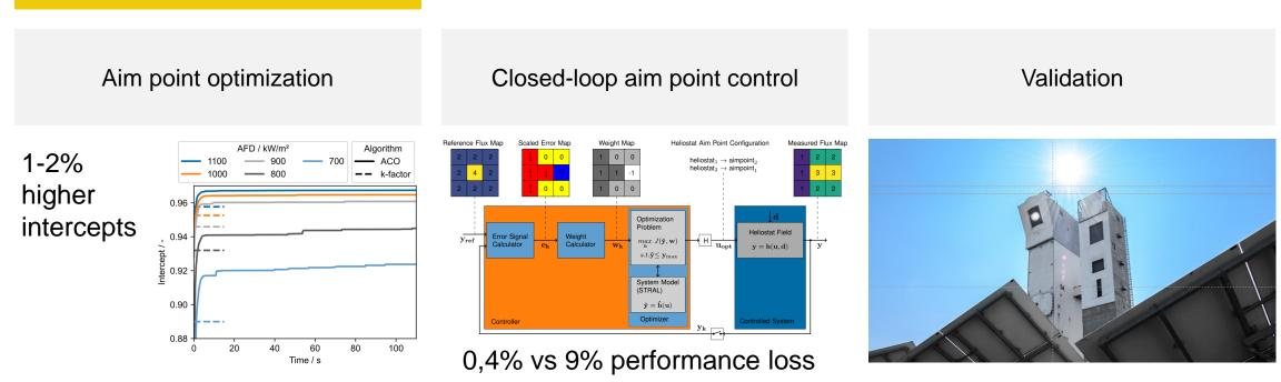
Additional yield of 1% amouts to 600.000 €/a for a 100 MW<sub>el</sub>-plant
