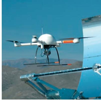
QFly – airborne collector shape measurement
