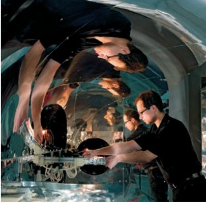
Linear solar simulator for receiver tests in the QUARZ laboratory in Cologne
