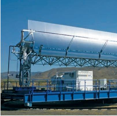
Rotating platform for performance testing of components at PSA
