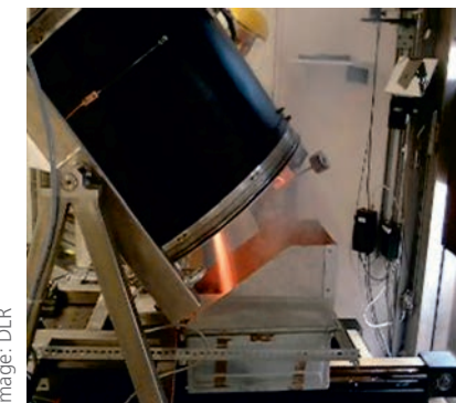
Aluminium being recycled in a rotating reactor
